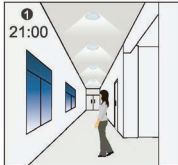
The light switches on at 100% when there is movement detected.
